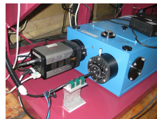
Ten-fiber bundle coupled to the spectrometer and imaged on the CCD, providing ten local measurements.
